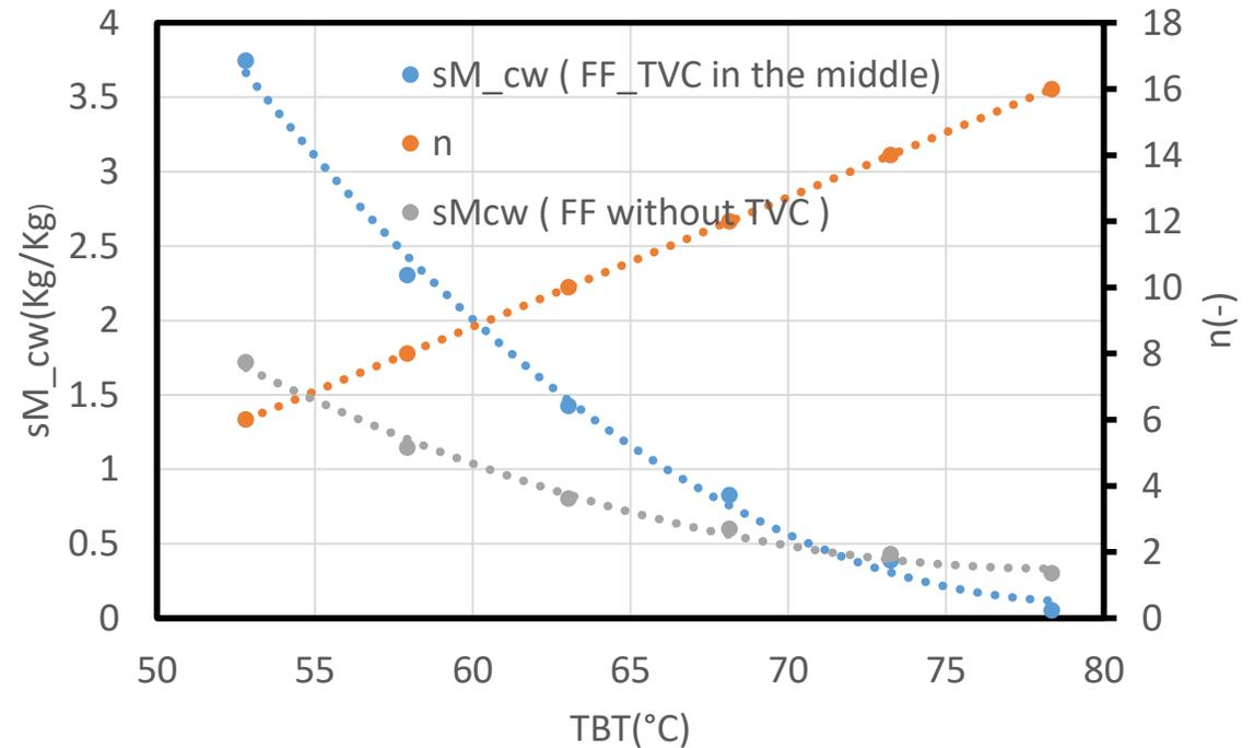
**Effect of increasing (TBT) on  $n$  and  $sM_{cw}$  for MED-FF system**
