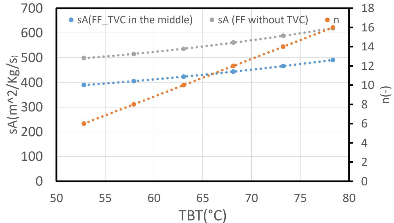
**Figure 4: Effect of increasing (TBT) on n and sA for MED-FF system**
