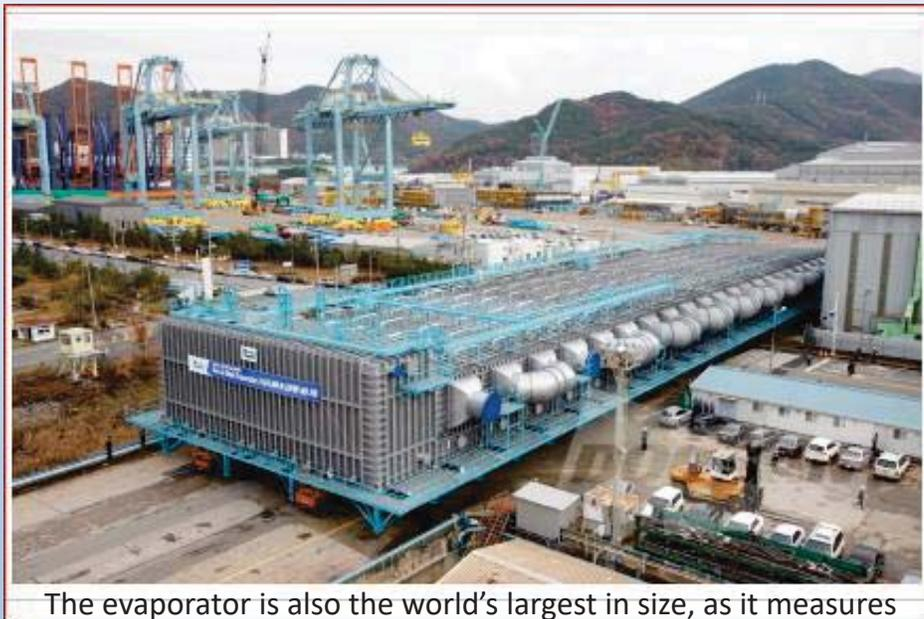
The evaporator is also the world's largest in size, as it measures 123 meters long, 33.7 meters wide, and weighs 4,150 tons
